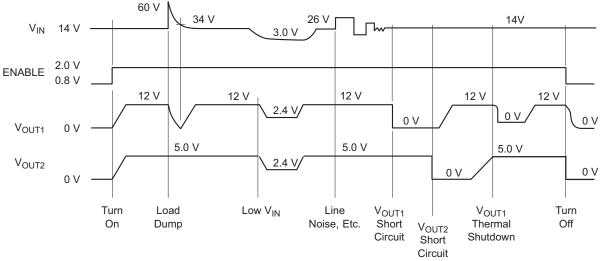
Figure 17. Typical Circuit Waveform
